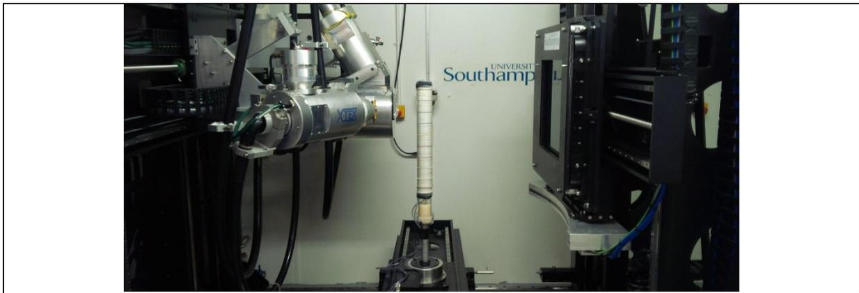
**Figure 1:**  $\mu$ -CT in-situ LCM experiment.
